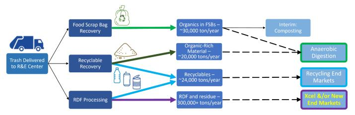
Over 330,000 tons of RDF are manufactured at the R&E Center annually, diverting this material from landfills. R&E holds an agreement with Xcel Energy (Xcel) for the management of RDF via combustion for electricity generation at two facilities. The fees the R&E Center pays to Xcel under this agreement equate to about \$6.5 million per year. The electricity generated from RDF is enough to power over 13,000 homes annually. This agreement expires on December 31, 2027.
