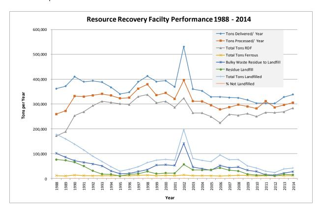
Through the processing of waste at the R&E Center, the R&E Board has prevented the need for 100 acres of landfill 40 feet deep. The prevention of this amount of waste going to a landfill has several environmental benefits including protection of groundwater and prevention of methane gas emissions. Additional social benefits include reducing long-term legal liability, avoiding the need to site a landfill in the Counties, and preserving available land for higher and better uses.
