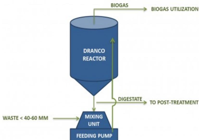
The MSW plants operate at a dry matter content in the digester of up to 40 %. In source separated organics and yard / food waste facilities, the waste is treated at a dry matter content of 20 to 35%. The company considers the strengths of the DRANCO process to include:
