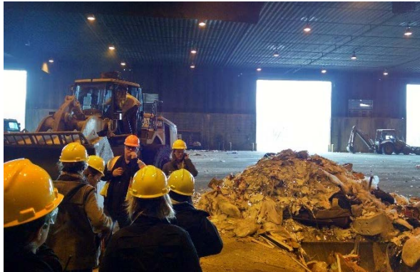
Figure J. The Recycling & Energy Center is a waste processing facility in Newport, Minnesota that shreds trash collected from homes and businesses to create fuel for energy.
