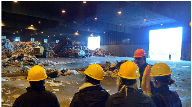
Figure 23. The Recycling & Energy Center in Newport, Minnesota shreds trash collected from homes and businesses to create fuel for energy as well as extracts metals for recycling.
