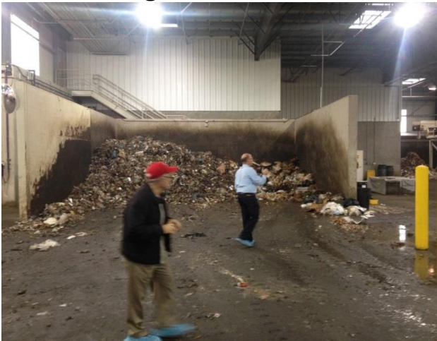
Photograph 1 is a bunker containing organics for the AD system in San Jose. These organics were recovered using MWP equipment.
