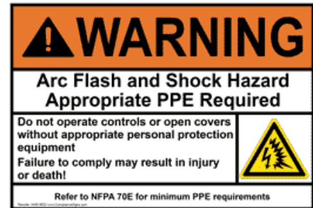
Picture 12-1 Arc Flash and Shock Hazard Warning Sign Source: www.compliancesigns.com
