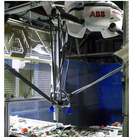
Picture 4-1 Robotic Sorter with a Suction Grabbing Mechanism
