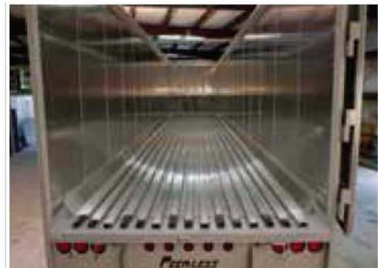
Picture 4-6 Hallco Live Floor™ "W" Floor Leak Proof Conveyor System Photo Courtesy of Hallco
